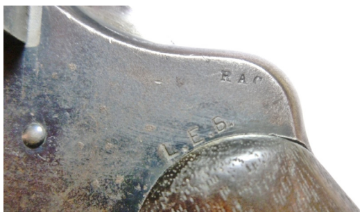
Figure 25: Note the inspectors proof marks on this military revolver or "martial gun." It is not a Colt SAA, but many Colt SAAs did have these stamps or "cartouches." The inspectors could be civilians or military ordnance officers proof-firing the revolvers. Their initials signify approval. The initials RAC are those of Rinaldo A. Carr. The initials L.E.S. are unknown.
