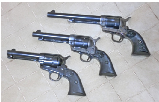
Figure 21: The most common barrel lengths, top to bottom: 7 ½ inches; 5 ½ inches; 4 ¾ inches. Other barrel lengths could be obtained by factory order. Note the hard rubber grips on the long-barreled revolver. It is a Type 2 eagle grip containing two profiles: on top, the trademark Rampant Colt, on bottom an eagle. The two bottom revolvers have the Type 1 hard rubber grip containing only the Rampant Colt. The original hard rubber grips issued in the 1880s were made of a substance called "gutta percha," an early type of latex.
