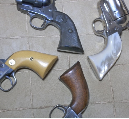
Figure 17: Various grips were available for Colt SAAs, some custom-ordered from the factory, others bought through after-market vendors. Since most revolvers were slightly different, grips (also called “furniture”) purchased from after-market vendors required careful fitting. Clockwise from top: factory hard rubber grips; pearlite grips, factory fitted on a 1961 nickel-plated .357 magnum; factory walnut grips on a U.S. Army martial revolver; real or faux ivory grips on a Second Generation SAA. Other grip styles will be shown in succeeding photos.
